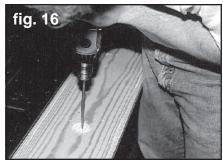
23. From the top surface of the boards, drill down through the 1/8" pilot holes with a 1/2" wood bit to complete the bed-to-frame mounting holes. See figure 16. Before drilling the hole, place a piece of scrap wood directly under the 1/8" hole to prevent splintering as the drill breaks through.
