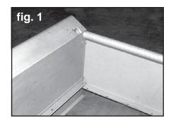
2. This bed requires the use of a long rod that attaches through the front bed panel top curl to the bed sides. Install a 5/16" flat washer, lock washer, and nut on one end of the rod. Insert the rod through the top hole in bed side into top curl of front bed panel.
