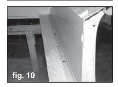
15. Attach the cross sills with brackets to the 5/16" bolts in the angle strips approximately 2-5/8", 26-5/8" and 52-7/8" respectively from the front bed panel. The two offset brackets go with the third cross sill from the front and the hole is offset toward the bed sides. Install lock washer and nut and hand tighten. The cross sills should be installed so that when the bed is installed on the frame the cross sills should be open toward the ground. See figure 11.
