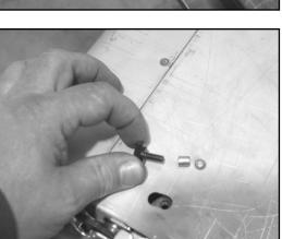
14. Bolt the link assemblies to each end of the tailgate. These are held in place by (2) ¼-20 x ¾" button head screws provided in the kit.
