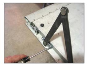
15. Lift the tailgate while directing the link assembly arms to the pivots attached to the bedsides. The link assembly arms will need to be folded in the upward direction for this. Lift the assembly until the slot in the link will fit onto the pivot.
