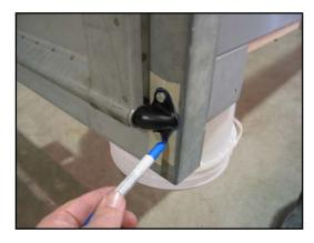
4. Remove the hinge marked in step # 3 above and remove the tailgate. Install the hinge back into position using the marked masking tape as a guide.
