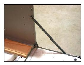
17. Raise the tailgate slowly making sure that the links fold downward this time. Close the tailgate slowly while checking for any interference. The latches will make a double clicking noise when latched slowly. Release the latches to check their operation. It may require slight inward pressure on the tailgate to release the latches.
