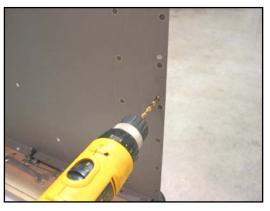
8. Using the 5/16-18 button head screws, install the latch strikers in the upper hole on each bedside. The latch striker can be held with a 9/16" wrench while tightening the button head screw.
