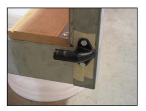
5. Slide the template provided onto the hinge far enough that the template can lay flat against the inside of the bedside. The outer edge of the template should be even with the outer edge of the bedside. Clamp the template in place. The template has been painted a dark color for the photo.
