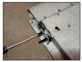
13. The latches are released by a black knob provided in the kit. Each of these black knobs needs to have an aluminum threaded spacer fitted to it. Thread the spacer onto the knob completely and then thread the knob into the tailgate latch through the slotted hole.
