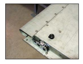
14. Bolt the link assemblies to each end of the tailgate. These are held in place by (2) 1/4-20 x 3/4" button head torx screws provided in the kit. Use a T27 torx driver to tighten these screws.
