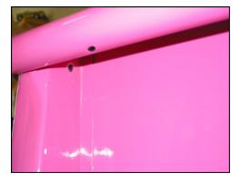
through. Use grommets and sleeving protect the wires from chaffing against the edges of sheet metal.
