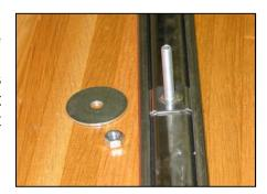
3. There may be a bed strip bolt in each space between cross sills that requires a 1-1/2" outside diameter washer with a 1/4" hole. This washer bridges the gap between the boards on the bottom and is placed on the bolt before installing the lock washer and nut.
