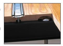
6. Bed strips with hidden fasteners for the 1953-1956 Ford flaresides will not have the front bed-to-frame hole punched in the strip.
