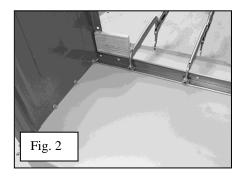
Note that the angle strip extends to the end of the bed wood at the rear sill, as shown in figure 3. If
