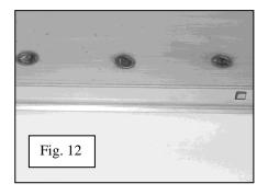
7. Grind the plug welds smooth and prepare for painting. See figure 13.
