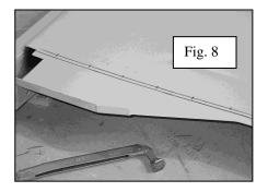
3. Mark three inch spacings along the length of the line drawn in step 2 to position the plug welds evenly. See figure 8. Drill a 1/4" hole through the bedside, not through the angle, at the location of each plug weld. See figure 9. Do not drill holes that go into the stake pocket cavity. Holes inside the stake pocket could not be welded. Deburr the holes to be sure there are no burrs that would hold the angle strip away from the bedside surface.
