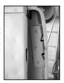
3. After the bracket is removed, clean up this area with a wire brush. There will likely be corrosion behind this bracket. Your bed side should now look like this. The two holes in the middle and the large rectangular hole will not be used. These holes will be covered by the new brackets from the other kits. They can be left open or welded shut.
