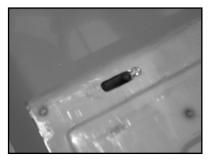
9. Install the spring on the plunger and slide it into the latch sleeve. A liberal amount of your favorite grease on the plunger is recommended before assembly.
