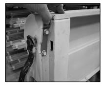
13. Once the latches are installed on both ends of the tailgate, re-install the tailgate on the truck. Make sure both latches are retracted and shut the tailgate. Hold the tailgate tight against the bedsides and release the latches by twisting the knobs. The latches have a pointed tip that will mark the bedsides for the rubber grommet to be installed.
