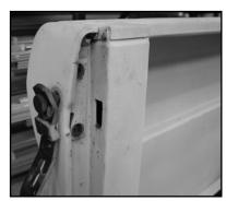
**Note:** If the brackets are welded to the bed side from the factory, You must drill and tap the original bracket to accept the grommet brackets. Place the grommet brackets into the upper corner of the bed sides. Mark the locations of the holes through the brackets. Drill and tap these locations to 5/16"-18. If you are not planning on using Mar-K's hidden link assemblies, you may also weld these grommet brackets in place.
