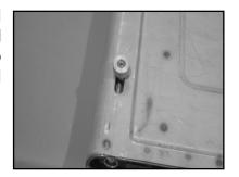
12. Remove the two bolts that hold the pivot bolt brackets to the upper portion of the bedsides. If yours are welded in, see the note below. It is not necessary to remove the brackets from the bedsides. Place the upper grommet brackets on top of these original brackets and re-install the bolts. Align the grommet brackets to the bedside outer profile and tighten these bolts. Due to the shape of these brackets, there is a left and right side and they will not fit if placed on the opposite bedside.
