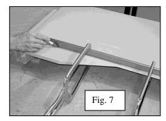
2. Remove the angle and draw a line the length of the bedside at the position of the plug welds, about 3/8" above the bottom of the angle strip. The welds should be midway between the bottom leg of the angle and the rolled edge of the top of the angle. See figure 8.
