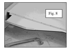
3. Mark three inch spacings along the length of the line drawn in step 2 to position the plug welds evenly. See figure 8. Drill a 1/4" hole through the bedside, not through the angle, at the location of each plug weld. See figure 9. Do not drill holes that go into the stake pocket cavity. Holes inside the stake pocket could not be welded. Deburr the holes to be sure there are no burrs that would hold the angle strip away from the bedside surface.
