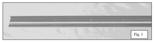
The angle must be installed with about 1/8" clearance between the front of the angle and the bedside flange that attaches the front bed panel. If the front bed panel is still attached, just allow 1/16" or less clearance between the angle strip and the front bed panel. See figure 2.
