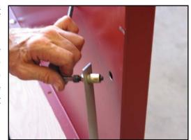
16. Supplied in the kit are 5/16"-18 shoulder screws and washers to act as upper pivots for the link assemblies. Place the bolts through the slotted end of the links. Then place the washer on the bolt. Thread these bolts into the threaded inserts. The washer keeps the link from scraping the bed side. Tighten these bolts with the 3/16" Allen wrench.
