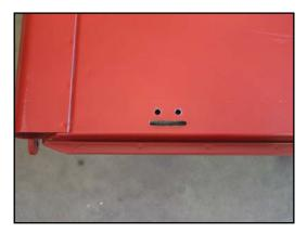
9. Insert the link assembly into the slotted hole. Attach the link assembly to the tailgate with two 1/4-20 x 3/8" button head screws. Tighten the screws with a 5/32" Allen wrench. It is important to notice that there is a left and right link assembly due to the pivot bracket of the link assembly. The offset part of the bracket where the rivet is should be at the bottom. This is the passenger side link shown installed.
