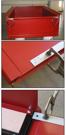
4. Mark the tailgate through the four 1/8" diameter holes in the template. Repeat this procedure for the other end of the tailgate with the same template. Make sure to flip the template over to get a mirror image pattern for the opposite side.
