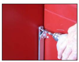
11. Lower and support the tailgate once again. Measure in from the back edge of the bed side 1-9/16" at the same vertical position as the drill mark and make a mark. Center-punch this position. Drill this position on each bedside with a 1/4" drill bit. Now drill this hole to a final size of 17/32".
