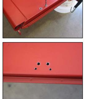
7. You need to cut a slot for the link assembly mounting bracket to fit through. Place masking tape on each side of the 3/16" diameter holes as shown. This will make it easier to see where to cut. Do both ends of the tailgate.
