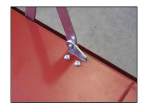
10. Now you need to position the upper pivot for the link assembly. Fold the link assembly as it would be when the tailgate is shut and lift the tailgate to the closed position. The link should be hanging vertical. Using a 3/8" diameter bit in a drill, place the drill bit through the slotted end of the link assembly as shown. Lift the drill bit to the top of the slot. Lightly drill the bedside with the drill bit just to leave a mark. Do this for both bedsides.
