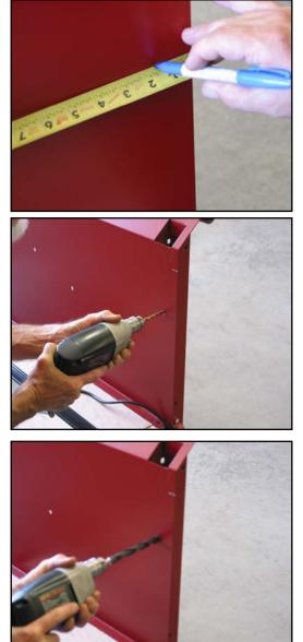
12. Test fit the threaded insert into the 17/32" diameter hole. Use a round file to enlarge the hole if the insert will not fit. Often, a drill will not make a perfectly round hole in sheet metal. Use the file to make the hole round. The insert must be installed so that its' flange is against the sheet metal surface of the bed side.
