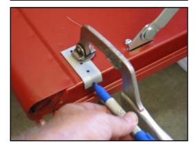
4. Center-punch the mark farthest in on the flat surface and drill a 3/16" diameter hole. You may want to use a drill stop so that the drill point does not damage the tailgate on the outside when it breaks through. Center-punch the other two marks and drill them with a 7/16" drill. It usually works better if you start with a small drill bit and work your way up to the 7/16" diameter.
