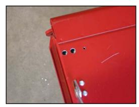
5. Place masking tape along the sides of the two 7/16" diameter hole to create a cutting guide as shown. Using a small high speed cutting wheel, connect the two 7/16" diameter holes by cutting the metal out between them. This will create the slot that the knob on the latch will slide in. Before finishing the second cut, grab hold of the scrap metal with pliers and keep it from falling inside the tailgate end.
