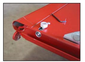
15. Insert the supplied rubber grommets into the bedside holes. Close the tailgate and release the latches into the grommets.
