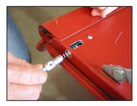
10. Push in on the plunger and position the aluminum knob with the stainless shoulder screw. Thread the screw into the plunger and tighten the screw with the 1/8" hex wrench.
