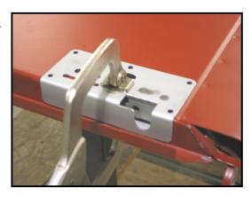
11. Bolt the rotary latch to the adapter panel by sliding the latch from the bottom up under the bracket as shown. Bolt the latch to the bracket with two 1/4-20 x 1/2" button head cap screws. Tighten the screws with a 5/32" Allen wrench.
