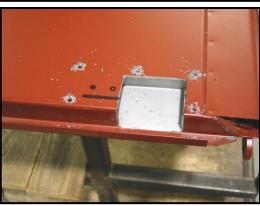
15. Center-punch the two larger marks and drill these with a 9/32" diameter drill. Center-punch the two ends of the area that will be slotted and drill these with a 7/32" drill. Cut the area of the slot out with a rotary tool with a reinforced cutting wheel. Place some masking tape along the edges between the holes to guide you. You can do this cutting with the high speed 3" tool, but you will have greater control with the smaller device.
