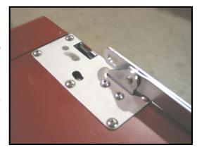
18. Thread the aluminum spacers completely onto the black knobs. Thread the knobs into the rotary latches through the slotted hole in the adapter panels. Check the operation of the latch. Lift up towards the top of the tailgate until the latch releases.
