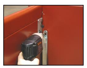
20. Lower and support the tailgate once again. Measure in from the back edge of the bed side 1-9/16" at the same vertical position as the drill mark and make a mark. Center-punch this position. Drill this position on each bedside with a 1/4" drill bit. Now drill this hole to a final size of 17/32".
