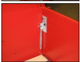
You have successfully installed the hidden latch and link assemblies. At final assembly, use a thread locking compound on all threaded areas to prevent them from coming loose.
