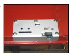
17. Slide the link assembly through the slot in the adapter panel and tailgate skin. Attach the link assembly to the tailgate with two 1/4-20 x 1/2" button head screws. Tighten the screws with a 5/32" Allen wrench. Note: It is important to notice that there is a left and right link assembly due to the pivot bracket of the link assembly. The offset part of the bracket where the rivet is should be at the bottom towards the tailgate hinge. This is the left (driver) side link shown installed.
