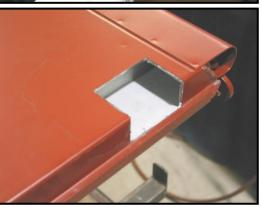
10. Remove the burs left by the cut-off wheel from the opening. Also make sure that the measurements are good. Refer back to step #3 & 4. Fit the adapter panel into the opening and check for clearance. The bottom of the adapter panel should be 10-11/16" from the bottom of the tailgate.
