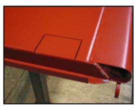
5. Create a vertical line on the edge of the tailgate from both horizontal lines. This marked area will need to be removed to allow the hidden latch to fit into the inside of the double wall structure of the tailgate.
