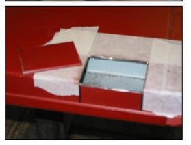
8. Cutting the vertical section of material away is a little harder. Rotate the cutting tool at an angle and move into the opening until you can cut all the way to the bottom of the vertical wall. The object here is to cut the vertical section without cutting through the outside flange of the tailgate. This outside flange is seen when the tailgate is closed and is not covered up by the adapter panel.
