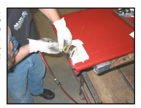
9. When you reach the bottom of the two vertical lines, Turn your tool back to flat but tilt it as shown. We need to cut along the bottom of the vertical sheet metal that is left. You will be leaving the strip of metal at the base that is spotwelded to the outside skin of the tailgate.
