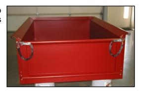
3. Support the tailgate in the horizontal (open) position. The tailgate has been removed in the photograph, but this is not necessary. Measure up from the bottom curl of the tailgate (15-1/2" for a 53-72 short bed) or (17-1/4" for a 73-87 short bed and 53-72 long bed) and make a mark. Using a combination square, draw or scribe a line 1-7/8" long inward towards the center of the tailgate.
