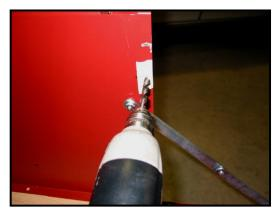
29. Bolt the strikers to the bedsides with the supplied 5/16-18 x 1/2" button head screws.
