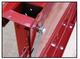
15. Raise the tailgate slowly to the closed position. The links should fold smoothly downward while closing. Supplied in the kit are two self-adhesive bumpers. Attach these bumpers where the link assembly will contact the tailgate when closed.
