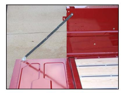
You have successfully installed the link assemblies. At final assembly, use a thread locking compound on all threaded areas to prevent them from coming loose. This kit is greatly complimented with our hidden tailgate latch which is Part # 130213.
