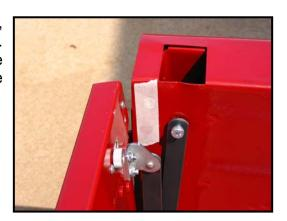
15. Release the latches by twisting the knobs. The latches have a pointed tip that will mark the masking tape for the position of the latch hole to be drilled in the bed side. Lower the tailgate and support it in the open position. Drill a 7/16" diameter hole. Again, it is better to start with a small drill and work up to the 7/16" diameter to ensure a more uniform round hole. If you have access to a step drill, these tend to make perfectly round holes in sheet metal.
