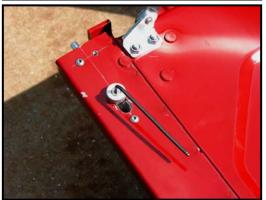
14. Once the latches are installed on both ends of the tailgate, make sure both latches are retracted and shut the tailgate. Hold the tailgate in a vertical position. Observe where the hidden latch plunger will hit the bed side when released. Place a strip of masking tape in this area.
