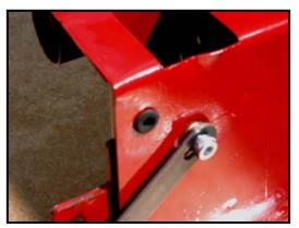
You have successfully installed the hidden tailgate latches. During final assembly, be sure to use a quality thread locking compound on all threads.
