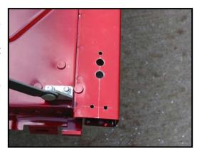
8. Place masking tape along the sides of the two 7/16" diameter hole to create a cutting guide as shown. Using a small high speed cutting wheel, connect the two 7/16" diameter holes by cutting the metal out between them. This will create the slot that the knob on the latch will slide in. Before finishing the second cut, grab hold of the scrap metal with pliers and keep it from falling inside the tailgate end.
