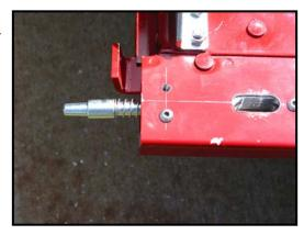
12. Push in on the plunger and position the aluminum knob with the stainless shoulder screw. Thread the screw into the plunger and tighten the screw with the 1/8" hex wrench.
