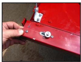
13. Test the movement of the plunger by sliding it back and fourth. Also pull the plunger all the way back and twist the knob to lock it in the retracted position. If the knob rubs on the tailgate or will not retract far enough to lock, you will need to enlarge the slotted hole in the tailgate with a file until full movement is obtained.
