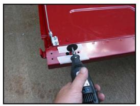
9. Clean up any burrs from the opening and straighten the sides of the slot if necessary with a file. Also clean up any burs on the inside of the curl where the drill bits and cutter broke through with a flat file. It is important that the latch barrel or sleeve sit flat against the inner curl of the tailgate.
