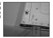
12. Once the latches are installed on both ends of the tailgate, re-install the tailgate on the truck. Make sure both latches are retracted and shut the tailgate. Hold the tailgate tight against the bedsides and release the latches by twisting the knobs. The latches have a pointed tip that will mark the bedsides for the rubber grommet to be installed.
