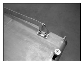
8. Now you need to position the upper pivot for the link assembly. Fold the link assembly as it would be when the tailgate is shut and lift the tailgate to the closed position. The link should be hanging vertical. Using a 3/8" diameter bit in a drill, place the drill bit through the slotted end of the link assembly as shown. Lift the drill bit to the top of the slot. Lightly drill the bedside with the drill bit just to leave a mark. Do this for both bedsides.
