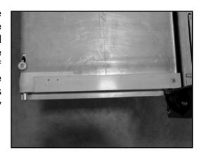
4. Mark the tailgate through the two 1/8" diameter holes in the template. Repeat this procedure for the other end of the tailgate with the same template. Make sure to flip the template over to get a mirror image pattern for the opposite side.
