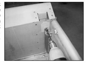
9. Lower and support the tailgate once again. Measure in from the back edge of the bed side 2-1/8" at the same vertical position as the drill mark and make a mark. Center-punch this position. Drill this position on each bedside with a 1/4" drill bit. Now drill this hole to a final size of 17/32".
