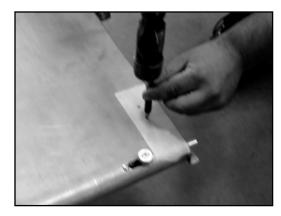
6. Drill the two holes on each end of the tailgate with a 1/4" drill.
