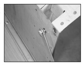
15. Raise the tailgate slowly to the closed position. The links should fold smoothly downward while closing. Supplied in the kit are two self-adhesive bumpers. Attach these bumpers where the link assembly will contact the tailgate when closed.
