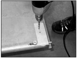
7. Attach the link assembly to the tailgate with two 1/4-20 x 1/2" button head screws. Tighten the screws with a 5/32" Allen wrench. It is important to notice that there is a left and right link assembly due to the pivot bracket of the link assembly. The offset part of the bracket where the rivet is should be at the bottom. This is the passenger side link shown installed.
