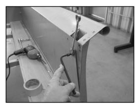
When repeating this procedure on the driver's side, the template will be positioned against the base of the bed side. Protect this area with a scrap piece of cardboard or wood. If you need further explanation of this procedure, go to <a href="https://www.mar-k.com">www.mar-k.com</a> and click on the Installation information on the home page. Scroll down to "Other helpful information" and click on "Threaded insert Information".
