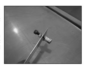
12. Place the insert into the hole in the bed side. Make sure to hold the insert flange tight against the bed side. Allow the template to rotate downward to the hinge area of the tailgate. This template will act as a handle to keep the insert from rotating when the nut is tightened.
