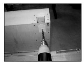
10. Test fit the threaded insert into the 17/32" diameter hole. Use a round file to enlarge the hole if the insert will not fit. Often, a drill will not make a perfectly round hole in sheet metal. Use the file to make the hole round. The insert must be installed so that its' flange is against the sheet metal surface of the bed side.
