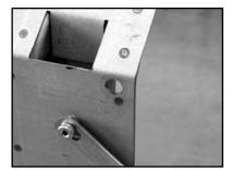
9. Insert the supplied rubber grommets into the bedside holes. Close the tailgate and release the latches into the grommets.
