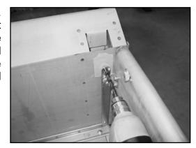
6. Lower and support the tailgate once again. Measure in from the back edge of the bed side 2-1/8" at the same vertical position as the drill mark and make a mark. Center-punch this position. Drill this position on each bedside with a 1/4" drill bit. Now drill this hole to a final size of 17/32".
