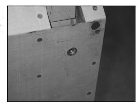
8. Special tools are available to squeeze the threaded inserts but we will show you how to do this without these special tools. Obtain the 5/16"-18 x 1-1/2" bolt and 5/16 hex nut supplied in the kit. Thread the hex nut about 1" onto the bolt. Place the bolt through the supplied flat washer and then through the 5/16" diameter hole at the bottom of the marking template. Next thread the insert onto the bolt with the flange of the insert towards the template finger tight against the template.
