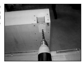
7. Test fit the threaded insert into the 17/32" diameter hole. Use a round file to enlarge the hole if the insert will not fit. Often, a drill will not make a perfectly round hole in sheet metal. Use the file to make the hole round. The insert must be installed so that its' flange is against the sheet metal surface of the bed side.
