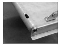
4. Install the spring on the plunger and slide it into the latch sleeve. A liberal amount of your favorite grease on the plunger is recommended before assembly.
