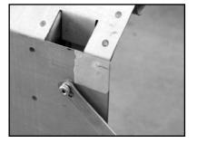
8. Lower the tailgate and support it in the open position. At each marked location on the bedsides, you need to drill a 5/8" diameter hole. Again, it is better to start with a small drill and work up to the 5/8" diameter to ensure a more uniform round hole. If you have access to a step drill, these tend to make perfectly round holes in sheet metal.
