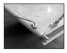
6. Test the movement of the plunger by sliding it back and fourth. Also pull the plunger all the way back and twist the knob to lock it in the retracted position. If the knob rubs on the tailgate or will not retract far enough to lock, you will need to enlarge the slotted hole in the tailgate with a file until full movement is obtained.
