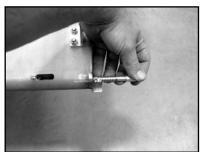
5. Push in on the plunger and position the aluminum knob with the stainless shoulder screw. Thread the screw into the plunger and tighten the screw with the 1/8" hex wrench.
