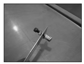
9. Place the insert into the hole in the bed side. Make sure to hold the insert flange tight against the bed side. Allow the template to rotate downward to the hinge area of the tailgate. This template will act as a handle to keep the insert from rotating when the nut is tightened.
