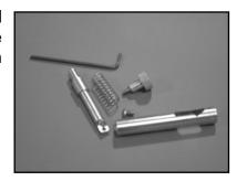
3. Slide the latch sleeve into the tailgate through the 5/8" hole until the small threaded hole lines up with the small hole in the tailgate. Thread the 10-32 button-head screw through the tailgate into the latch sleeve and tighten with the supplied 1/8" hex wrench. Check the alignment of the slot in the tailgate with the slot in the latch sleeve.
