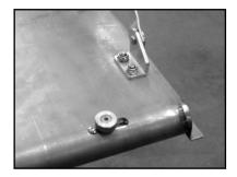
7. Place some masking tape onto the top rear corners of the bed sides as shown. Make sure both latches are retracted and shut the tailgate. Hold the tailgate tight against the bedsides and release the latches by twisting the knobs. The latches have a pointed tip that will mark the tape on the bedsides for the rubber grommet to be installed. If you have purchased Mar-K bedsides with the bedside upgrade for hidden latch & link proceed to step #9.
