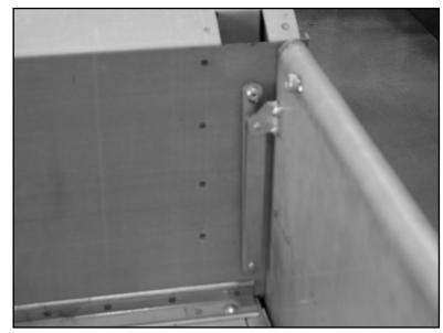
You have successfully installed the link assemblies. At final assembly, use a thread locking compound on all threaded areas to prevent them from coming loose. This kit is greatly complimented with our hidden tailgate latch which is Part # 100265 shown already installed.
