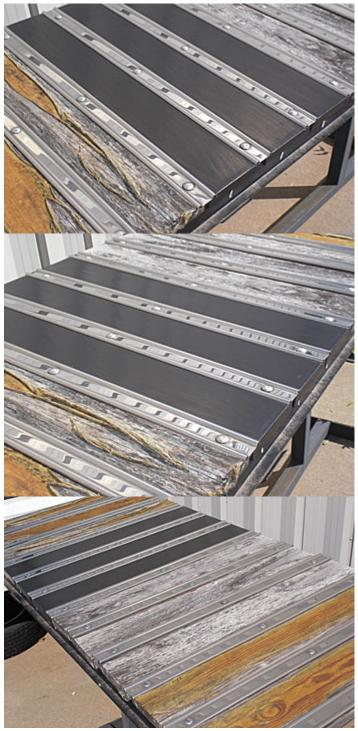
In summer 2007 we wrote the "final" test results for our second bed wood finish evaluations. At that time all the clear finishes had failed to some degree and only the painted samples had not failed. The original plan was to continue to monitor and report the results until all samples had failed. This is being written in summer 2010 and after 5 years continuous exposure to Oklahoma weather, the painted samples have dulled slightly but still have not cracked or separated from the wood.
