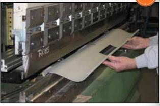
Rear Pans are formed in this press brake. Custom tools needed to make parts are designed and built at MAR-K™.
