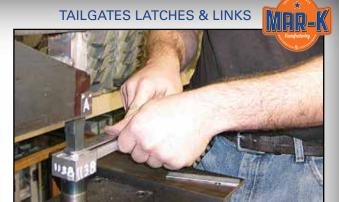
A MAR-K<sup>™</sup> employee attaches two link pieces to each other using this special pressing tool.
