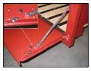
MAR-K™ now makes a kit for installing the hidden rotary style latches and link assemblies into a stock Ford tailgate. Adapter panel is made of 16 gage electro-galvanized steel and link assemblies are avail-
