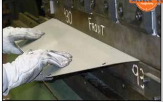
The top of MAR-K's<sup>™</sup> Fleetside Repair Panels is embossed with an offset using this CNC press brake.
