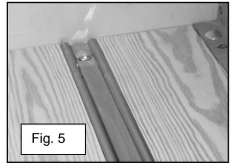
16. Insert the 5/16"-18 x 1-1/2" carriage bolts through all holes in the bed strips. A few of the bolts will not line up with anything. These bolts will get a 1-1/2" outside diameter washer on the bolt before the lock washer and nut. This bridges the gap between the boards on the bottom side. See figure 6.
