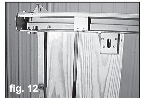
mark should be **93-1/8"** from the center of the mark to the front of the wood near the front bed panel.
