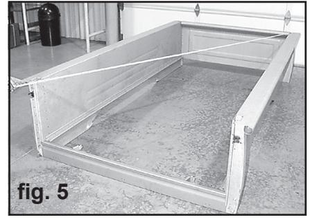
7. Place the assembly on supports horizontally to gain access to both the top and bottom of the bed floor area.
