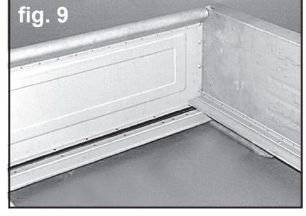
13. Place the next board into position on both left and right hand sides leaving approximately a 1/2" gap between the boards.
