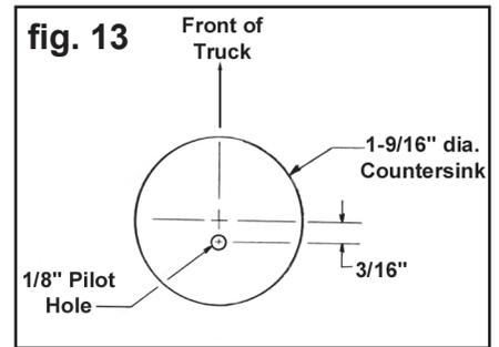
22. On the top surface of the boards, measure toward the front of each board 3/16" from each pilot hole and mark the boards for the countersink. See figure 13.
