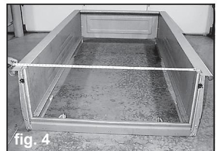
6. Measure crosswise from the front of the bed to opposite rear of the bed on both sides. See figure 5. These measurements should be within 1/16" of each other to ensure bed squareness. Now tighten all bolts.
