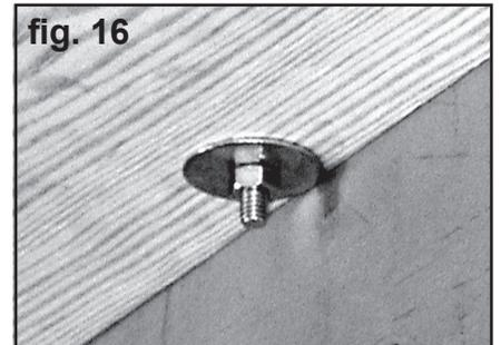
26. There are two other sills that are similar in appearance to the cross sills only smaller. These reinforcement strips attach to the bed strip bolts approximately **36-13/16"** and **57-1/16"** from the front bed panel.
