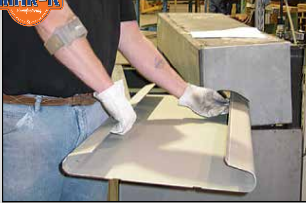
Electro-galvanized steel is bent to the correct curve on a MAR-K™ tailgate.
